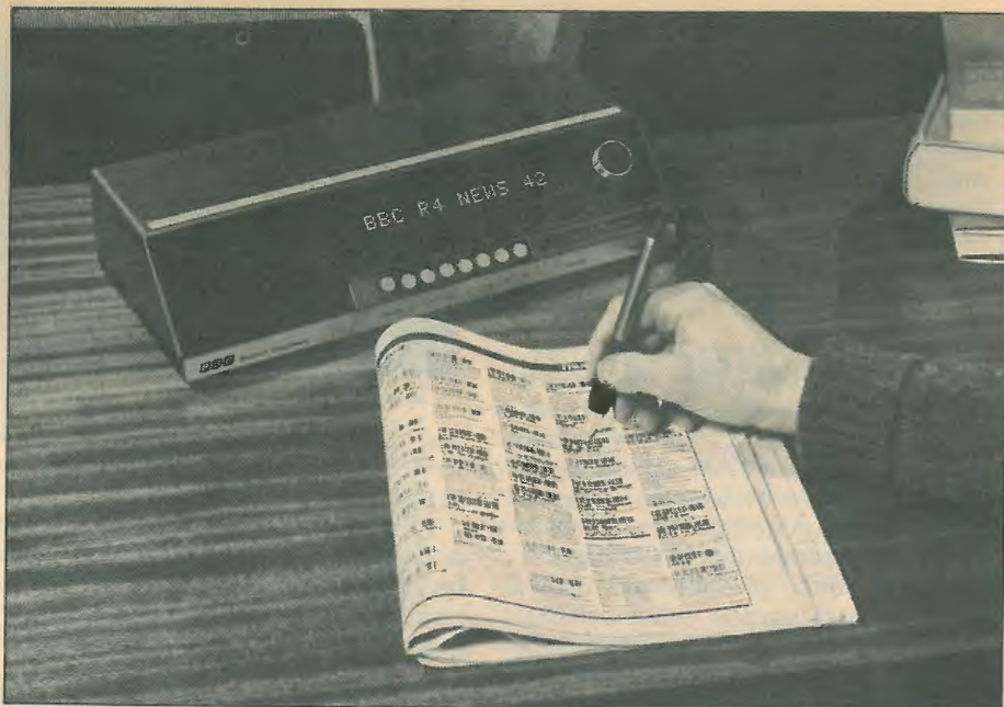
Experimental BBC radio receiver allows programmes to be selected digitally by a sensing pen drawn across bar codes printed in the Radio Times.
