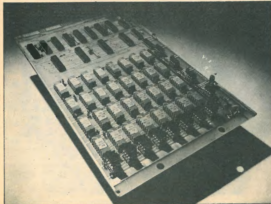
2Mbit television field store based on c.c.d. devices, as used in digital standards converter and digital noise reducer. ▼
