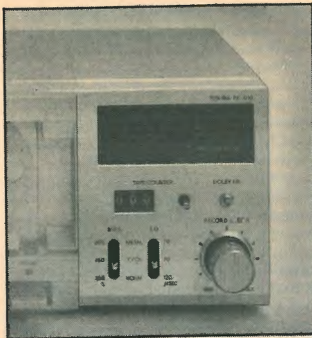
Cassette recorders for the 'eighties will have bias and equalization for metal-particle tape but will the public pay the extra price?
