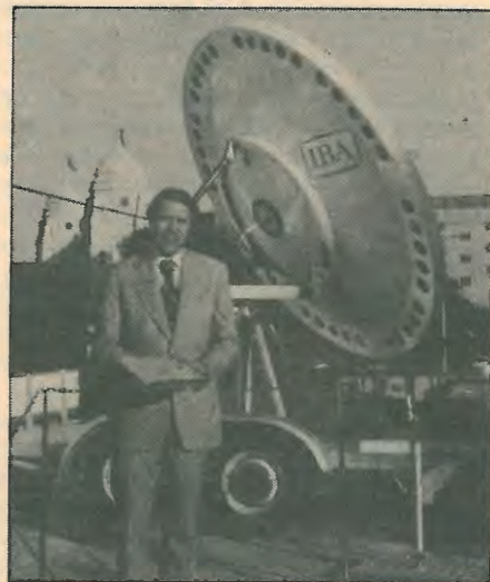
IBA's transportable 14GHz up-link to OTS satellite used for ITN broadcast from Wembley conference centre.
